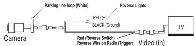
1) Find a suitable location to flush mount install the camera. Make sure the camera's view is unobstructed and be careful not to drill into any wires that might damage the vehicle, also check to make sure you have enough depth for install. When all connections have been made and before mounting the camera, verify the camera is working and has good view of the area. Use the supplied 28mm hole saw bit to drill a hole for flush mounting of camera, then install camera.
