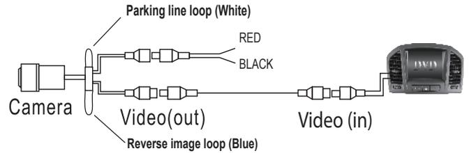
1) Find a suitable location to flush mount install the camera. Make sure the camera's view is unobstructed and be careful not to drill into any wires that might damage the vehicle, also check to make sure you have enough depth for install. When all connections have been made and before mounting the camera, verify the camera is working and has good view of the area. Use the supplied 20mm hole saw bit to drill a hole for flush mounting of camera, then install camera.
