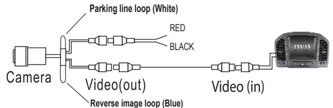
1) Find a suitable location to flush mount install the camera. Make sure the camera's view is unobstructed and be careful not to drill into any wires that might damage the vehicle, also check to make sure you have enough depth for install. When all connections have been made and before mounting the camera, verify the camera is working and has good view of the area. Use the supplied 20mm hole saw bit to drill a hole for flush mounting of camera, then install camera.
