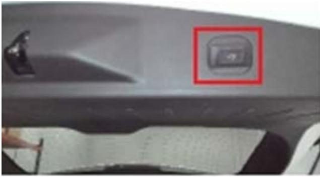
14. Use the provided hole saw to drill a hole for the rear button and mount it using the provided hardware.
