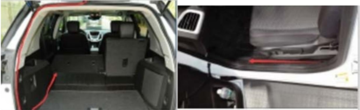
10. Run the wiring to the front of the vehicle for the remained of connections.
