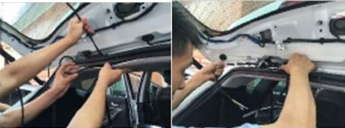
9. Route the wiring for the power through the boot of the tailgate using a threading tool.
