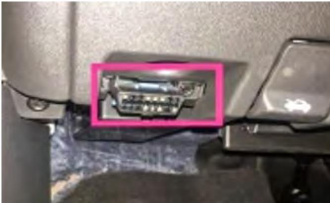
8. Using the provided t-harness, replace the OBDII harness with the provided connectors and install the t-harness in line with the vehicle harness.
