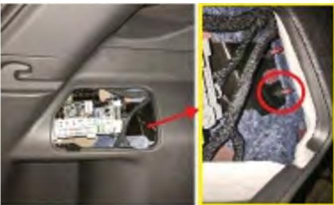
13. There is a rear grounding wire on the harness. Above is the suggested location of the ground, but any clean chassis ground location can be used.
