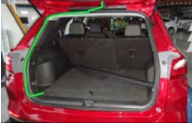
14. Run the wiring to the tailgate of the vehicle. Wiring will need to go through to boot of the tailgate for a clean looking install.
