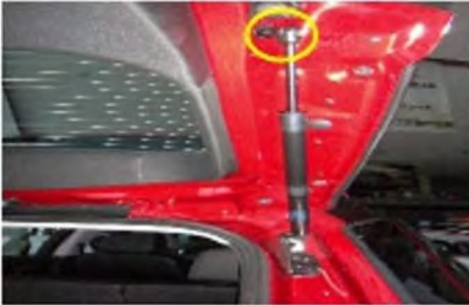
2. Remove the factory struts from the left and right.
