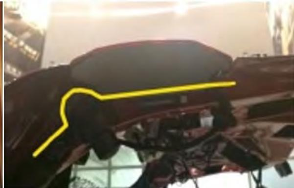
5. A hole will need to be drilled for the power strut wiring. A 16mm hole is suggested. Please measure out the wire and drill carefully to avoid internal wiring and components. Take notice to the closing positioning before drilling, the wire from the powered strut should not get caught between the vehicle body and tailgate when closed. A grommet is provided on the wire to provide a water tight seal.
