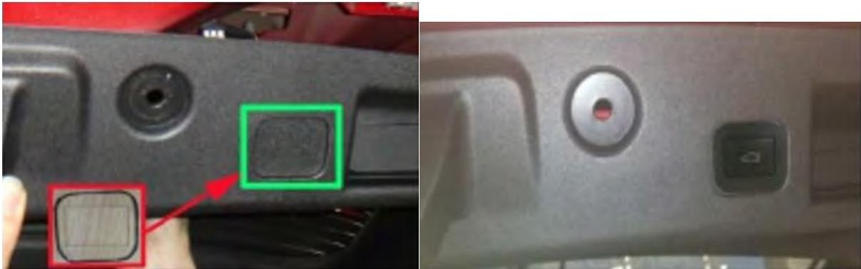
15. To mount the rear button, use the clear template plate provided with the kit to trace out an outline for the button on the tailgate panel. Then mount the rear button as show in the photo.
