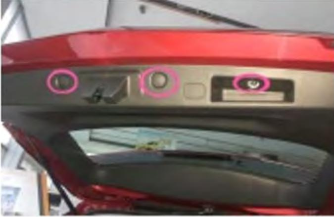
1. Remove the screws in the locations shown in the picture and remove the panels from the tailgate.
