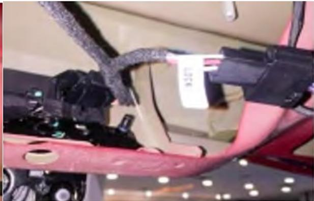
6. Install the provide t-harnesses in line with the factory wiring for the locking and electronic opening mechanisms. Also find a good location in the tailgate for the buzzer. Buzzer attaches with double side tape.
