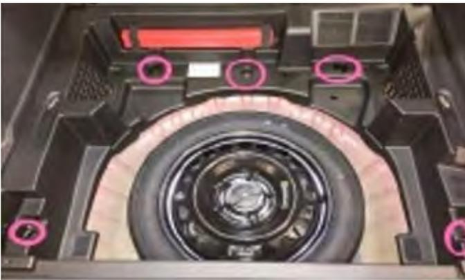
12. Removing the rear of the vehicle may help with running the wiring to the tailgate. Remove the screws in the locations shown in the photo to remove the plastic panel.
