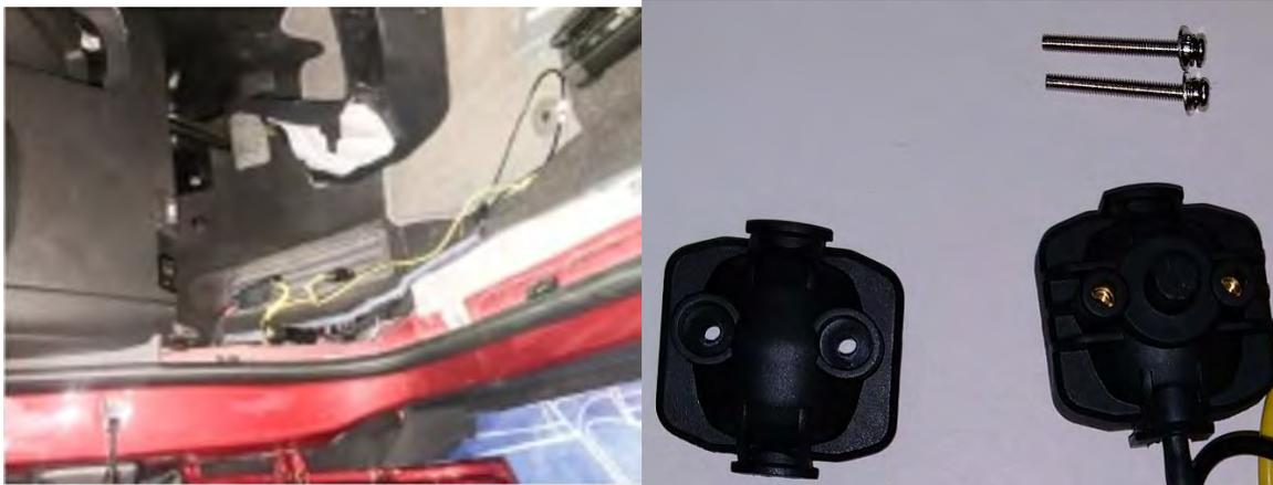
10. Using a digital multi-meter find a reliable 12 volt constant source and using the provided wire clamp tap into the 12v wire.
