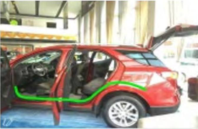
11. Run the wiring from the front of the vehicle to the rear in the direction shown in the photo.
