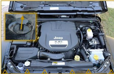
2. Lean grille forward. Using panel pry tool, release the metal clips.
