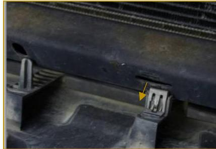
3. Unclip turn signal by rotating it out of socket. To removing signal, push plastic retainer inward to release, pushing housing out of grille.
