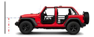
• To create your X-axis (horizontal) line, make a straight-line using tape by connecting the center points between the headlights.
