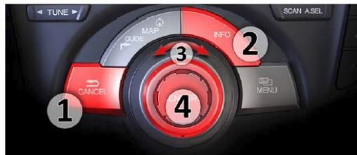
**Step 1:** Switch to the video source by holding the CANCEL button (1) for three seconds.
