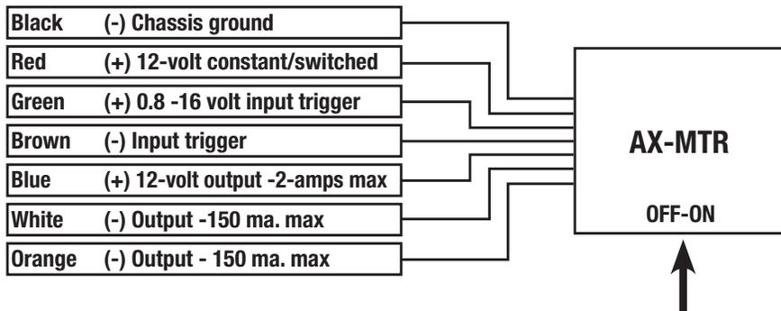
Programming switch must be turned off after the AX-MTR is programmed!
