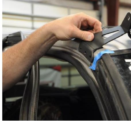
5. Remove the mounts from the truck and drill the previously marked holes with a  $\frac{1}{4}$ " drill bit making a pilot hole.
